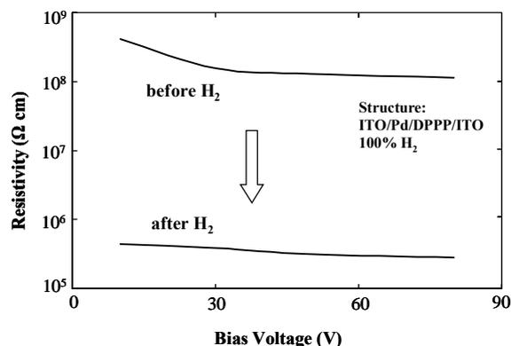
Fig. 5: Change in resistivity of the sensor.
