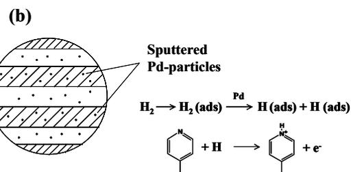
Fig. 3: (a) Interdigital electrodes and (b) magnified Pd-sputtered electrodes.
