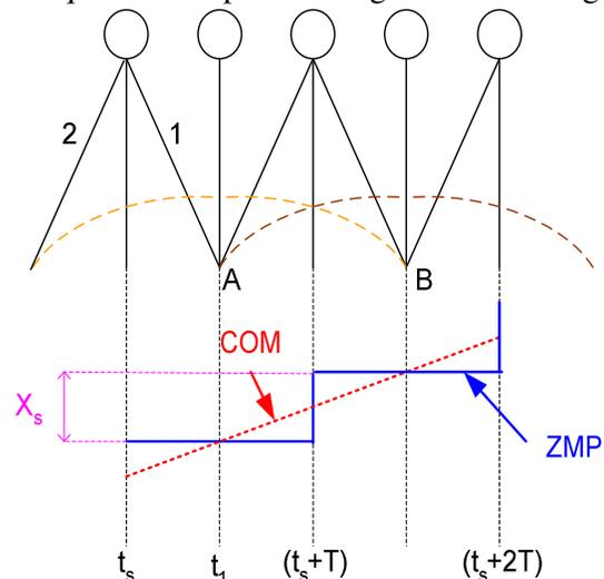
Figure 1: Requirement of ZMP and COM movement while biped walks
