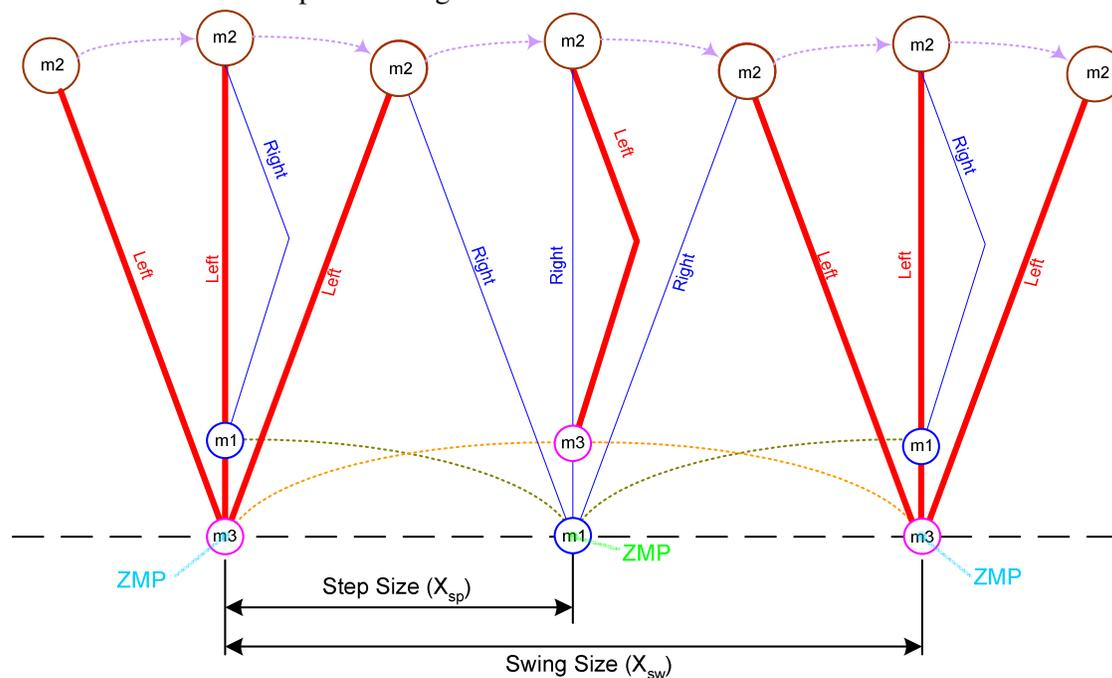
Figure 3 : The walking process( Three mass biped)
