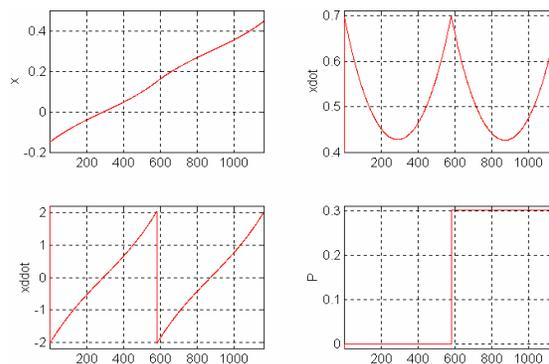
Figure 2 : Analytical trajectories solution (one mass biped- hip moving horizontally)
