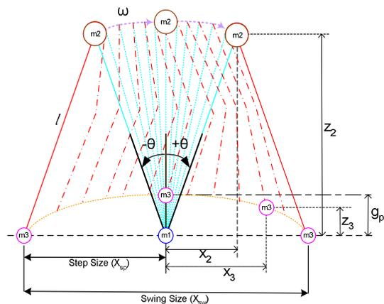
Figure 4: Hip and swing leg motion( Three mass biped)
