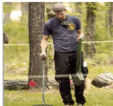
Fig. 5 Metal detector being used in landmine detection
