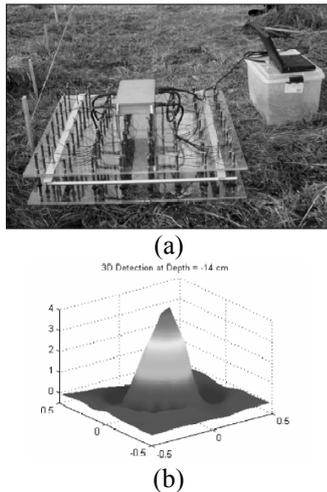
Fig. 9 EIT Landmine Detector and results
