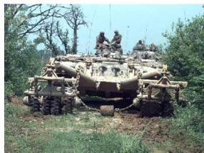
Fig. 16 Panther armoured mine clearing vehicle
