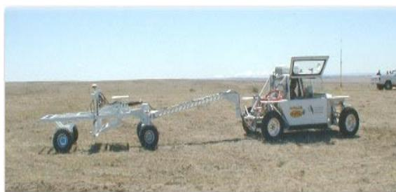
Fig. 3 Unmanned vehicle based landmine detection – Scheme 2
