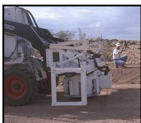
Fig. 13 – Thermal Neutron Activation Sensor
