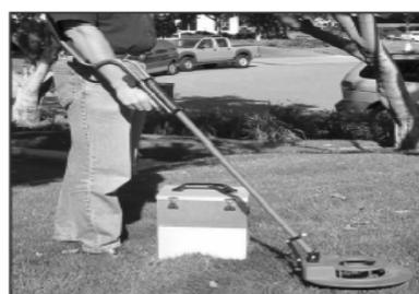
Fig. 7 – Prototype NQR Handheld Mine Detector
