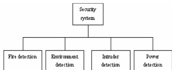
Figure4 The security system architecture
