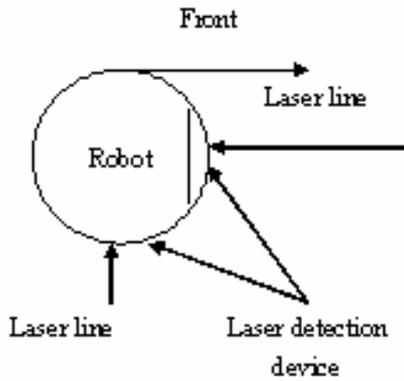
Figure 9. the auto-recharging method for LCSR-I
