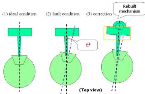
Figure 11. an error angle  $\theta$  in the docking situation
