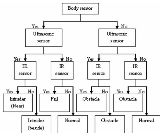
Figure5. The detection rule of the intruder system
