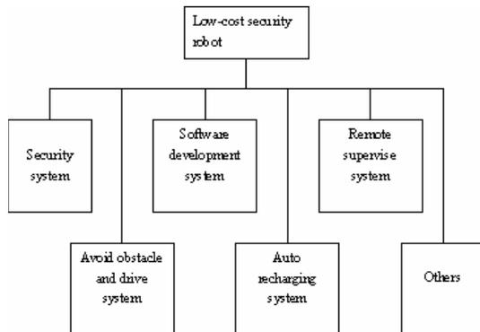
Figure 2. The hierarchy structure of the security robot.
