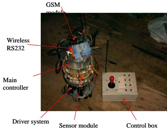
Figure 1. The contour and structure of intelligent security robot.
