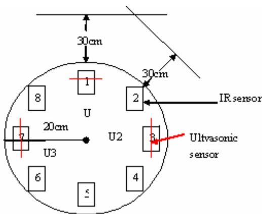
Figure7. the arrangement of IR and ultrasonic sensors
