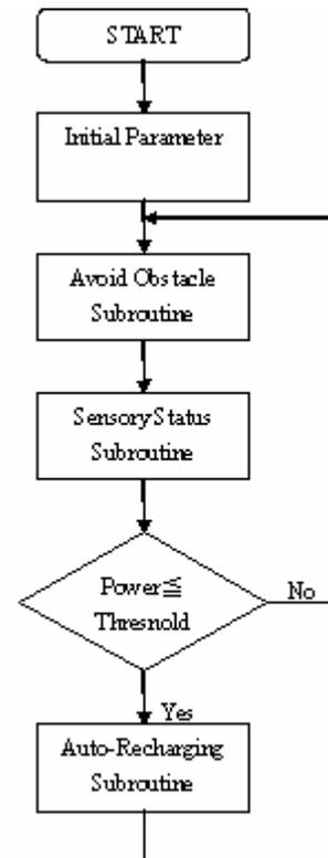
Figure 8. The software flow chart for the low cost security robot
