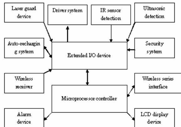
Figure3 The hardware architecture of the robot
