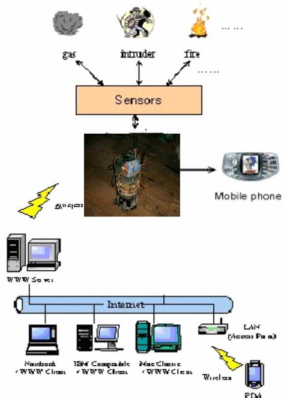
Figure 6. The hardware configuration of the remote surveillance and control architecture.
