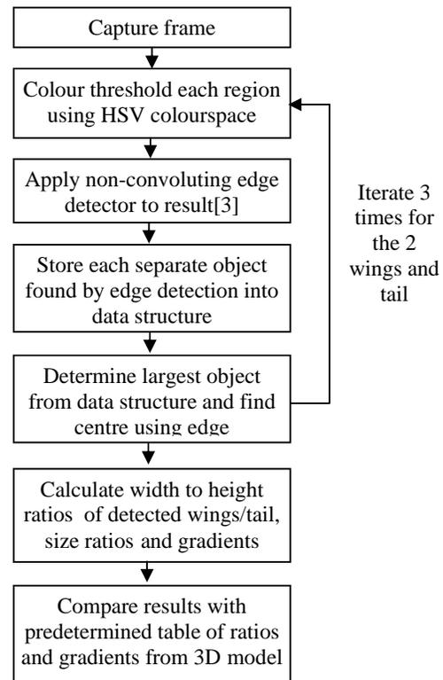
Figure 4 Attitude Determination Software Model
