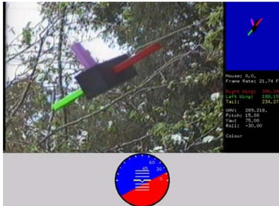
**Figure 5** Testing the In-Flight Attitude Determination System with model airframe in real lighting conditions.
