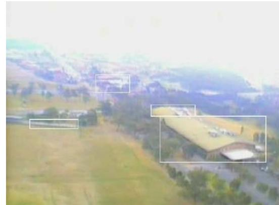
**Figure 6.** Actual footage from a UAV with the possible unnatural objects detected
