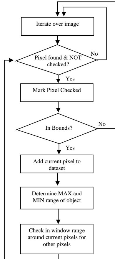
**Figure 9.** Recursive search algorithm for natural/unnatural object detection
