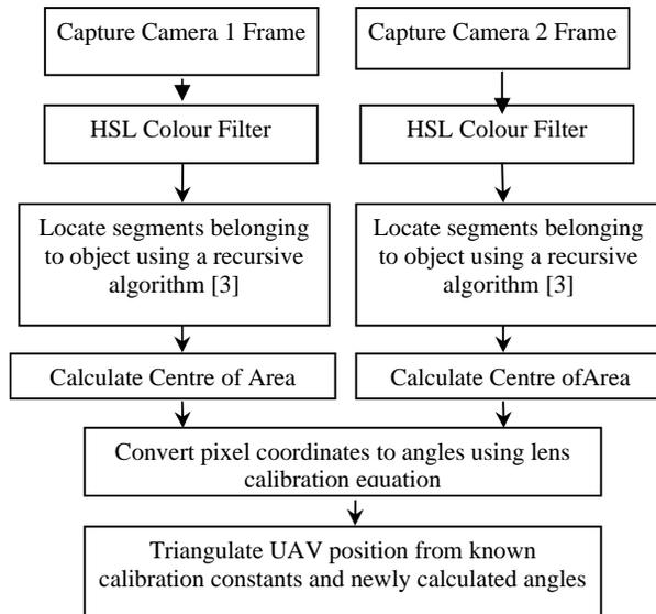
Figure 2. LAAS Software Block Diagram
