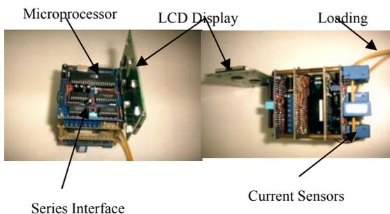
Figure 6. The on-line detection and diagnosis modular.
