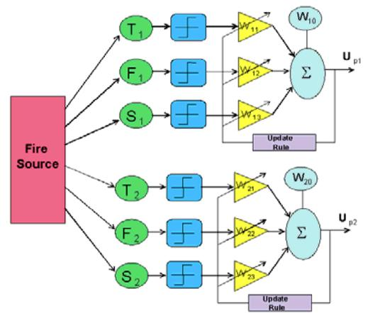
Figure 3. Adaptive multisensor fusion architecture
