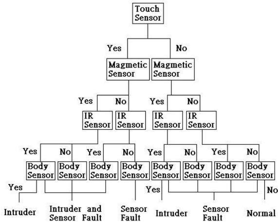
Figure 4. The detection and diagnostic rule of the intruder system
