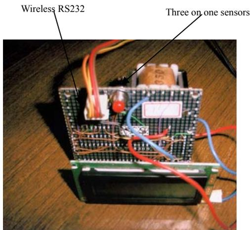
Figure 5. The fire detection modular
