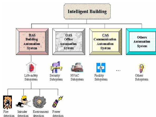
Figure 1. Intelligent Building Architecture
