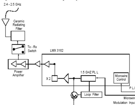
Figure 2 : Transmitter Block
