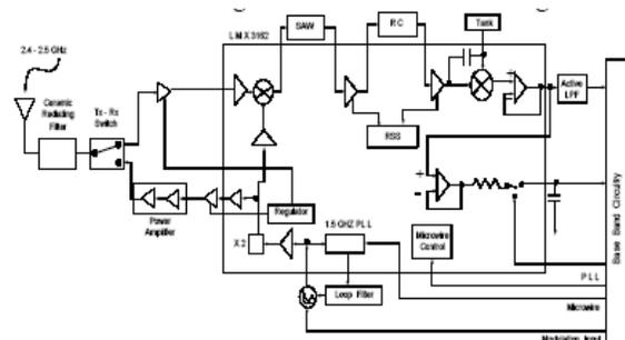
Figure 1 : Transceiver Blocks Synthesizers
