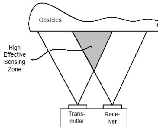
Figure 6 : High Effective Sensing Zone
