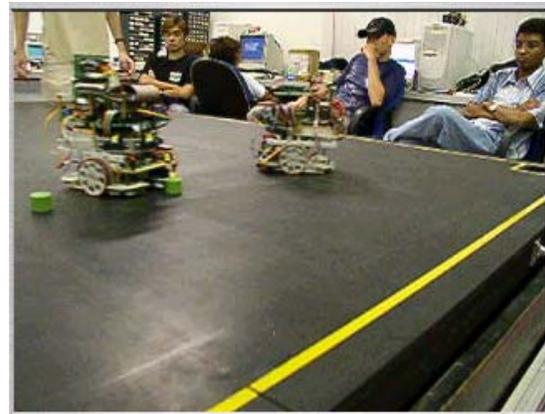
**Figure 5:** Robot pair collaborating to dispose all the pellets on the board to designated locations.
