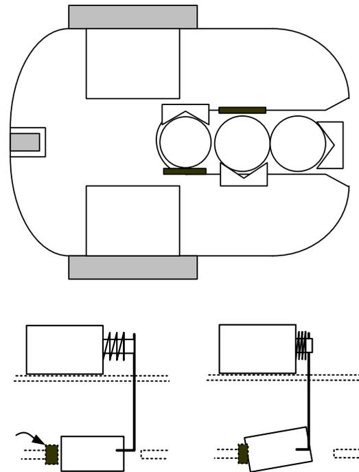
**Figure 1:** Robot chassis and the grabber mechanism.
