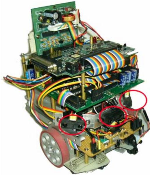
**Figure 2:** A picture of the robot. Highlighted areas show the position of proximity sensors.
