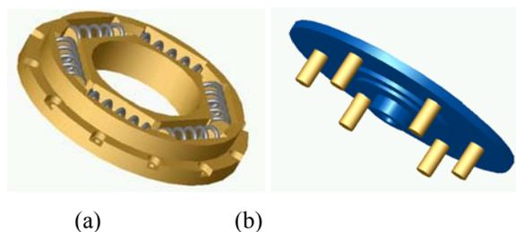
Figure 7: A three-dimensional model of the spring component: (a) lower part, (b) upper part.
