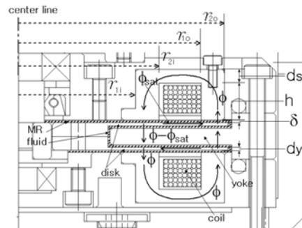
Figure 2: A sectional view of the damper for explaining fluxes in the case that current flows in both coils.
