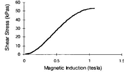
**Figure 4:** Shear stress versus magnetic flux density of the MRF-132LD [10].
