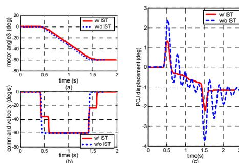
Figure 13: vibration reduction for 3<sup>rd</sup> axis:
