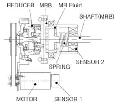
Figure 1: Design of passive compliant joint mechanism.
