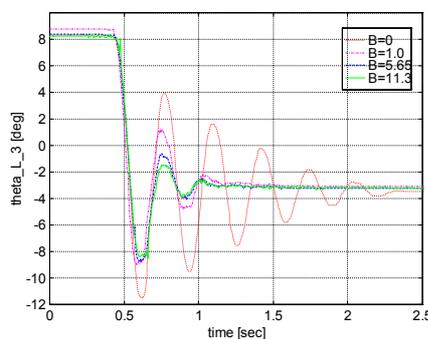
Figure 10: Damped results according to change of  $B$ .
