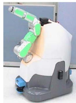
Figure 8: The developed safe arm and mobile robot.
