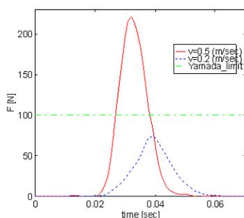
Figure 12: Measured impact forces.
