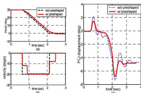
**Figure 15:** Experiment: vibration reduction for 2nd axis: (a) motor angle of the 2nd joint, (b) command velocity of the 2nd motor, (c) displacement of the 2nd PCJ
