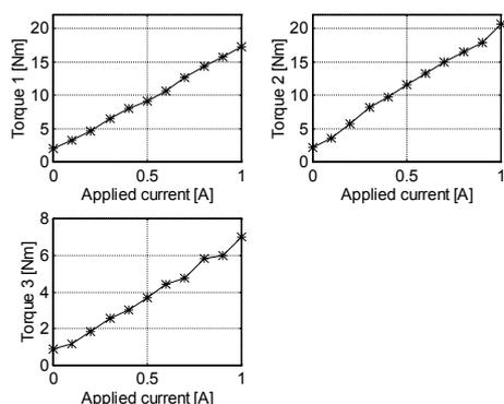
Figure 6: Relations between generated torques and applied currents of the MR dampers.
