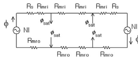
Figure 3: A magnetic circuit considering saturation effects.
