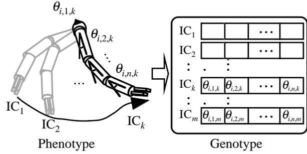
Figure 7: The representation of the  $i$ th trajectory candidate composed of  $m$  intermediate configurations
