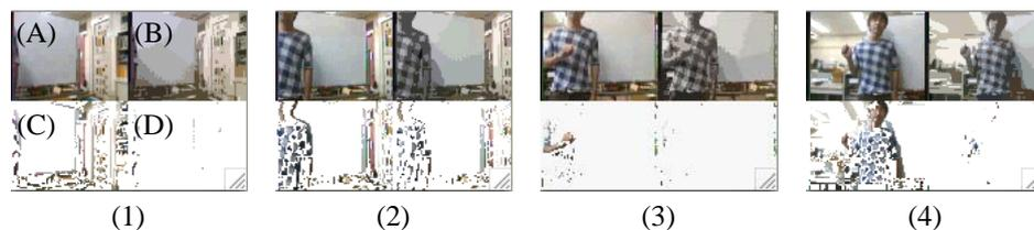
Figure 9: An example of visual tracking: (A) an original image, (B) reduced color image, (C) difference between two images, and (D) moving objects by the differential extraction.
