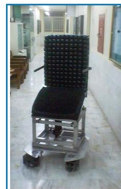
**Figure 7** Fabricated prototype of robotic nurse unit, Mechanical structure.
