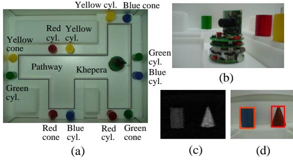
Figure 2: (a) An experimental world. A total of 12 objects, which are two each of red, blue, green and yellow cylinders and one each of red, blue, green and yellow cones, are arranged as landmarks. (b) A Khepera robot. (c) A saliency map. (d) Attended spots.
