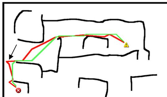
**Figure 10:** The sequence of gates are not always along the actual (green) optimal path, this leads to generate a path with less distance optimality.
