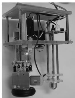
**Figure 3:** Photograph of the Horizontal Wheel Driving Mechanism
